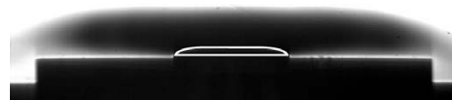
Fig. 5. Schlieren image of the vapor layer above an evaporating hexane film from the level substrate geometry. The liquid film is outlined by the white lines.
