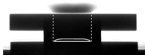
Fig. 7. Schlieren image of the vapor layer above an evaporating hexane film within a well of depth 9.7 mm. The white dashed lines outline the interior of the well and the white solid lines outline the liquid film.
